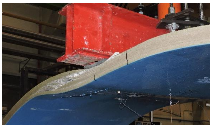
Figure 7 – Full-scale tests: interlaminar shear with delamination of the different layers.
